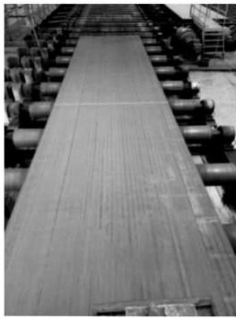
图 1 NM450 钢淬火后板形 Fig. 1 Plate shape of NM450 steel after quenching
